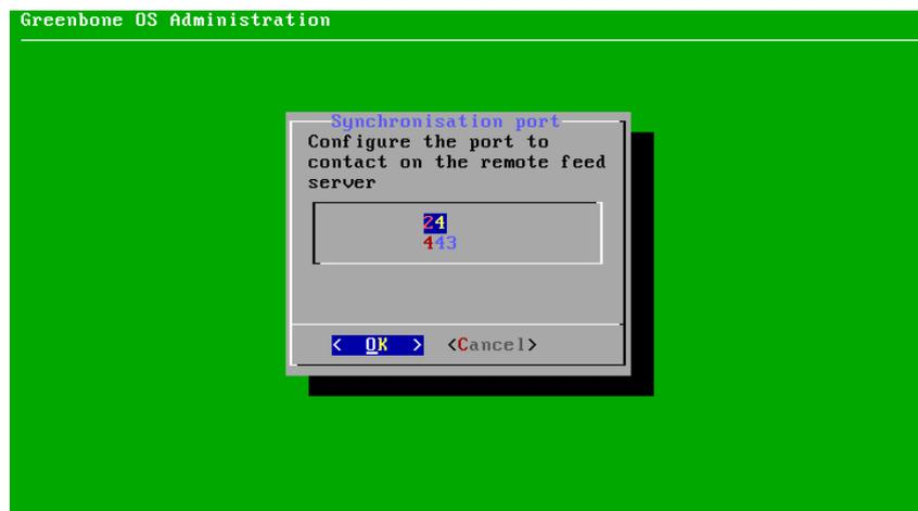
Fig. 6.33: The sync may use either 24/tcp or 443/tcp
